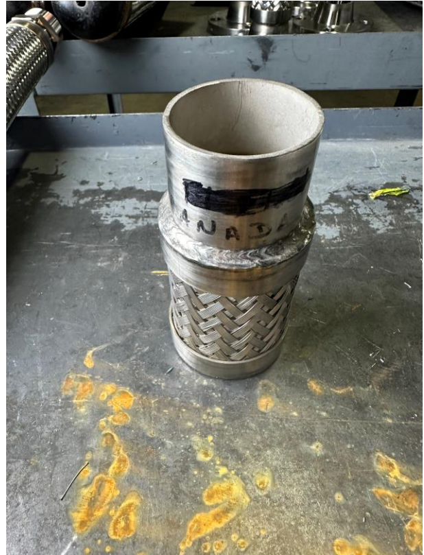
Discoloration (left) and a “V” pattern in weld bead (right) are examples of poorly executed fitting attachment welds.
