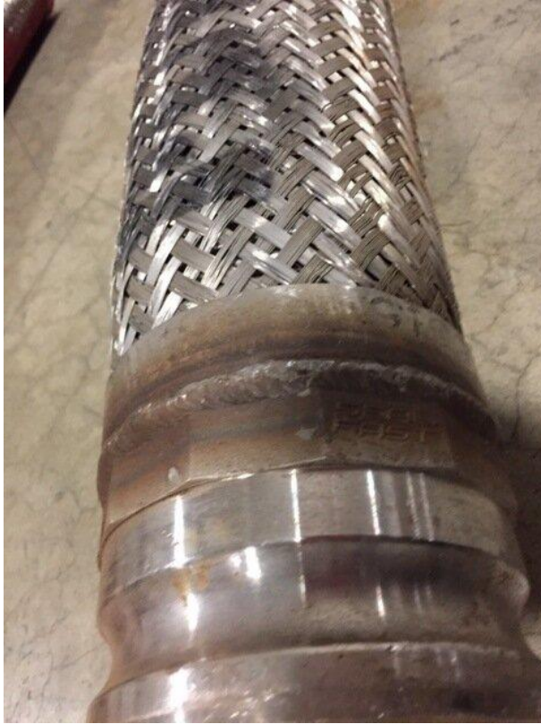
Discoloration (left) and a “V” pattern in weld bead (right) are examples of poorly executed fitting attachment welds.
