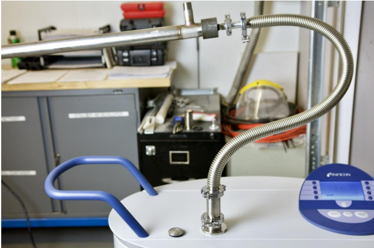
Figure 1: Mass spectrometer machine pulling vacuum on chamber containing hose assembly.
